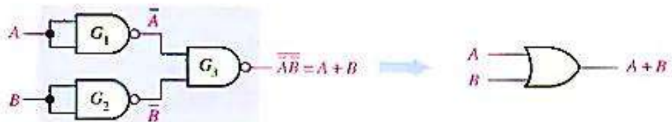
(c) Three NAND gates used as an OR gate
